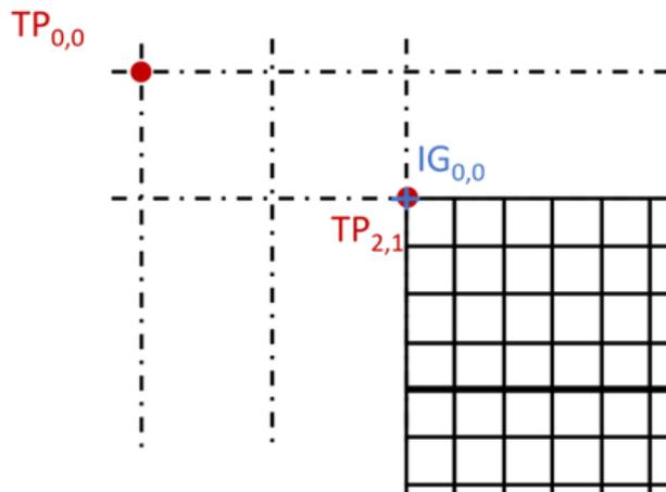
This means that  $TP_{0,0}$  in the image above has these offset values assigned. The tie-point  $TP_{2,1}$  will be located at the upper-left corner of the first image pixel  $IG_{0,0}$ .
