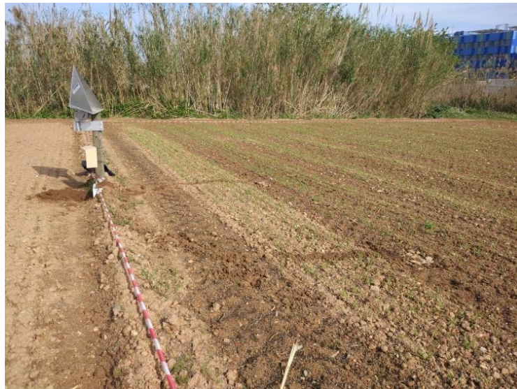
Figure 8.1 The triangular trihedral of 50 cm edge used for calibration in the barley campaign
