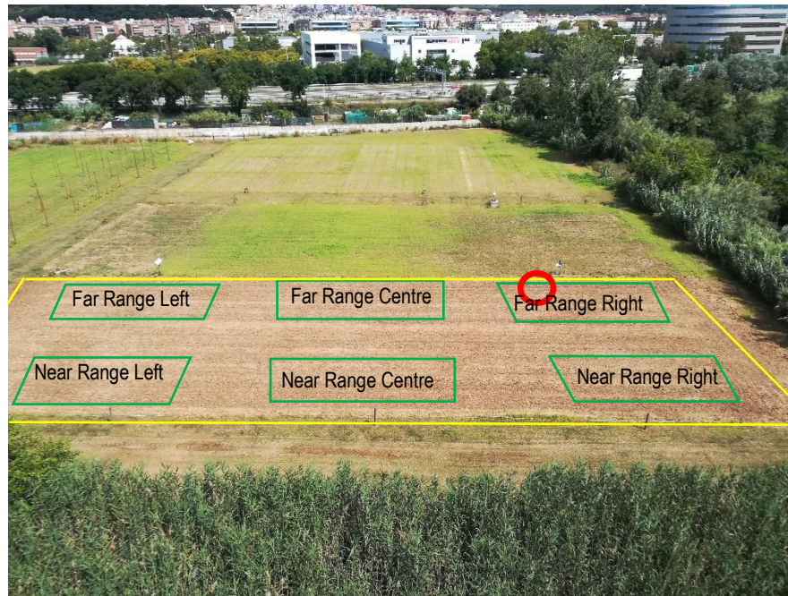
Figure 6.8 Position of the EC-5 sensors (red circle). Sensors were placed 4 meters from the contour of the field, on the right, in Far Range.
