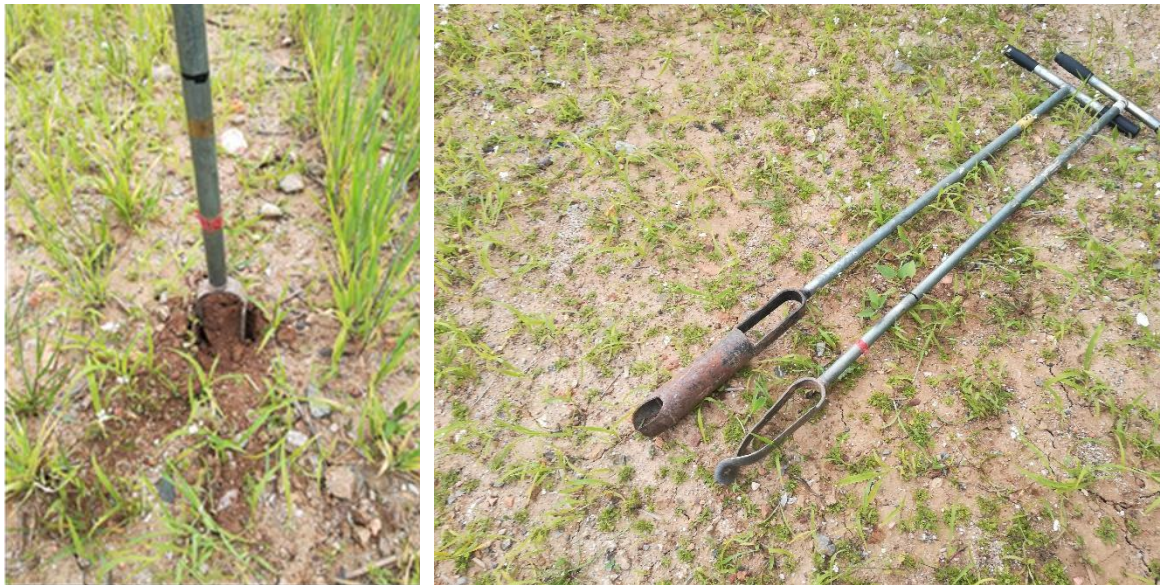
Figure 6.11 T-Style Samplers used to take samples for Gravimetric Soil Moisture determination
