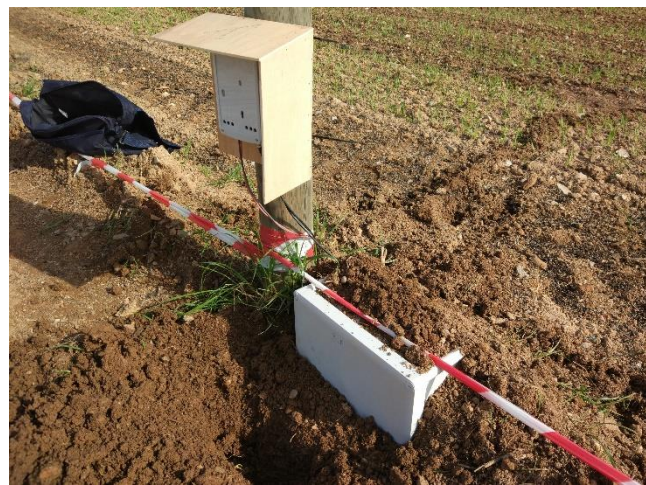
Figure 6.7 Photographs of the soil moisture and weather parameter Logger installed in Far Range
