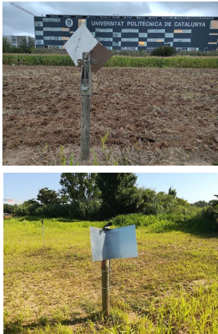
Figure 8.2 A triangular trihedral with a 50 cm edge, a vertical dihedral and a 45° tilted dihedral, made of two 40x40 cm 2 metal plates, were deployed in the field in the corn campaign. The trihedral was relocated to a centred position in front of the field
