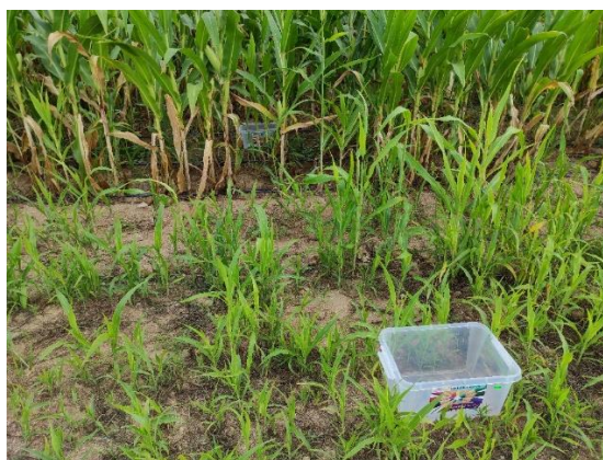
Figure 7.13 Interception of precipitation. Two buckets were strategically deployed to measure the intercepted precipitation by comparing the accumulated water.
