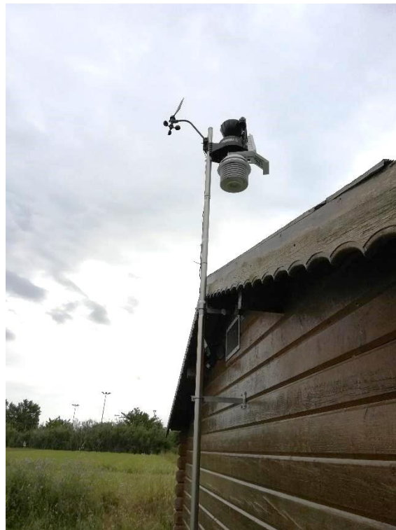
Figure 6.20 A local Weather Station (DAVIS Vantage Pro 2) was installed next to the test field
