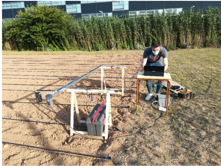
Figure 7.2. Soil Roughness was measured, as in the barley campaign, by means of a Laser ranger on a rail. The Profile length was 2.1m with a sampling interval of 2 mm. Different locations of the field were measured with different rail orientations.
