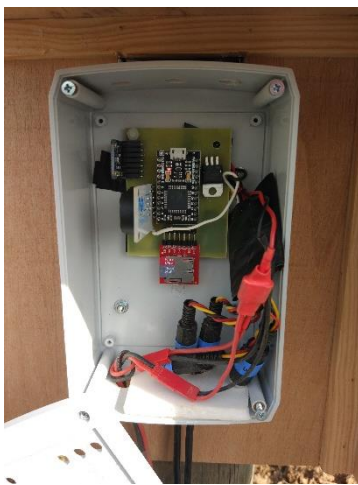
Figure 6.7 Photographs of the soil moisture and weather parameter Logger installed in Far Range
