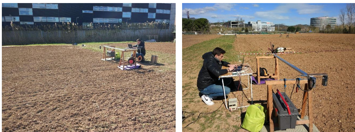
Figure 6.3. On 6 March 2020 soil Roughness was measured by means of a Laser ranger on a rail. Profile Samples were taken every 2 mm, at different positions of the field
