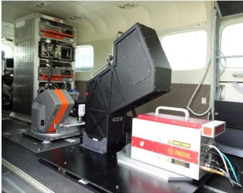
Figure 13: TASI-600 and laser scanner (LiDAR) Riegl LMS-Q780 mounted in the aircraft together with the *HyPlant* sensor.
