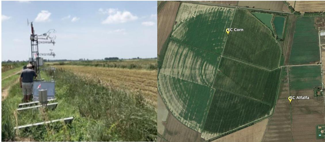
Figure 19: Left side: EC station with vertical wind profiles and net radiometer installed in the corn area at Le Rogaie site (Italy). Two EC stations were installed in Le Rogaie on two different crops (corn and alfalfa) for all the duration of the experiment. Right side: Localization of the EC stations at Le Rogaie site (Italy) in 2018.
