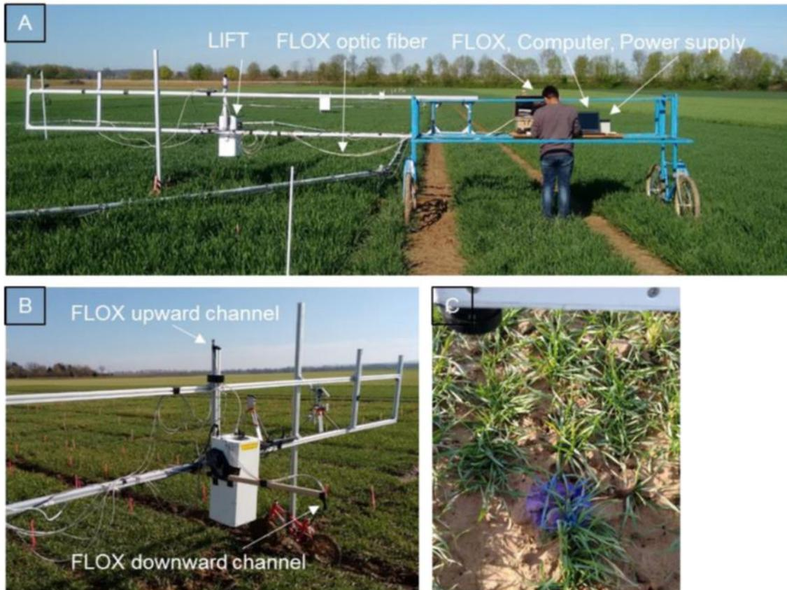
Figure 121: Manual position system Field4Cycle modified for Breedface measurements, mounted with the LIFT and FloX device, (A) where FloX upwelling and downwelling fibers were placed such to avoid shading (B) and the blue light excitation area (approx. 3 cm in diameter) is shown in the shade covering multiple wheat leaves.
