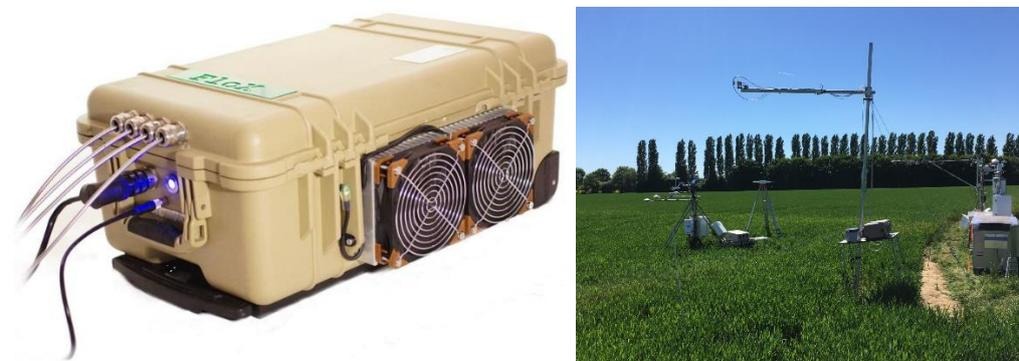
Figure 14: The FloX system. (Left) The temperature controlled and sealed central unit of the FloX system with the four-fiber optics that collect incoming and upwelling radiance on the two spectrometers. (Right) The FloX system as it is installed in a winter wheat field in Selhausen. The fiber optics are placed in the NADIR position about two meters above the canopy, continuously collecting light for fluorescence retrieval.
