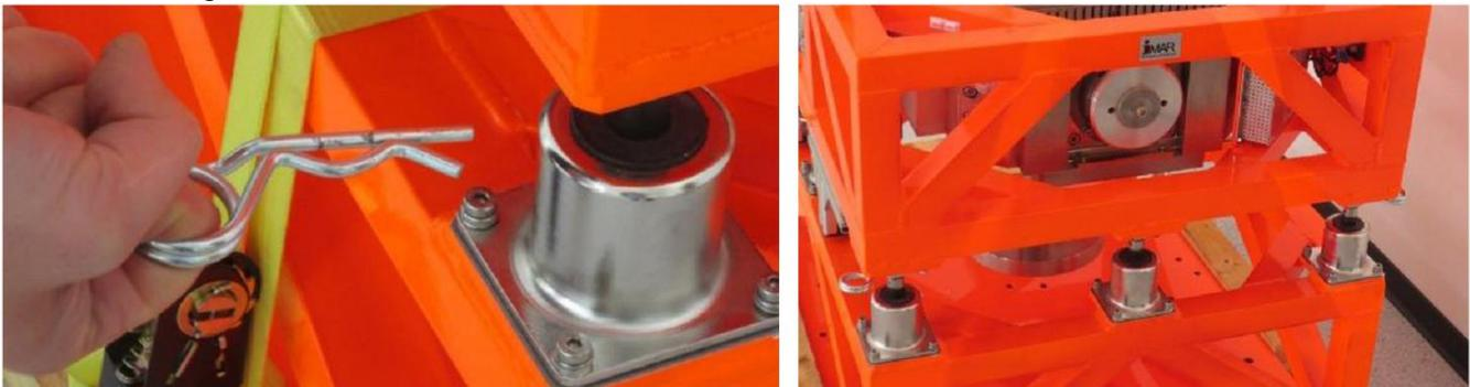
Figure 4 - Vibration isolators of the platform.
