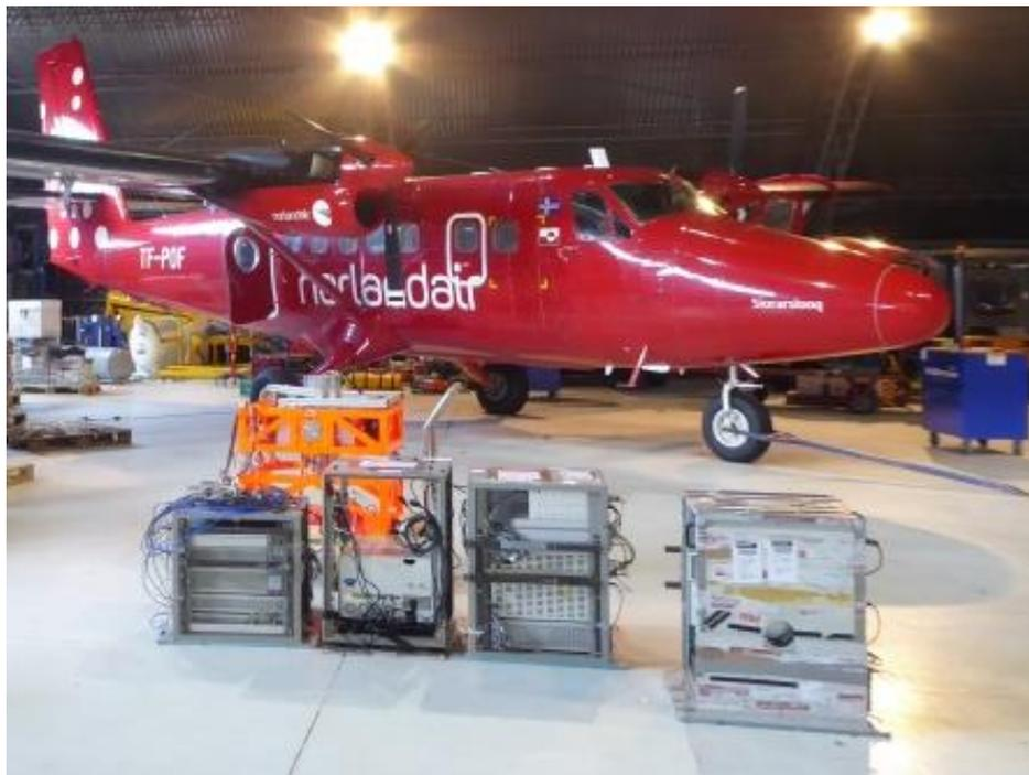
*Figure 10 - Gravimeter packaged for airplane installation. On the front, one can see the four cabinets containing the electronic and laser racks of the gravimeter.*
