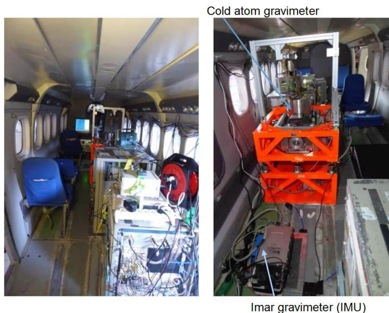
Figure 12 - Picture of the installation of the gravimeter in the airplane.
