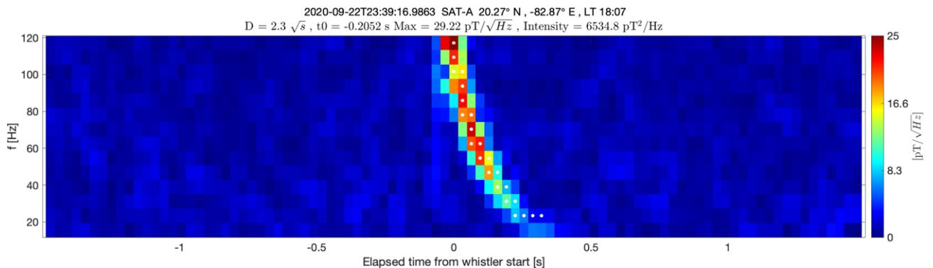
Figure 5-4 Example of whistler characterization for time and intensity parameters. The tiles on the PSD plot that are crossed by the dispersion curve are indicated by white dots. They are used to compute  $t_0$ , its uncertainty and the intensity of the whistler in this frequency range.
