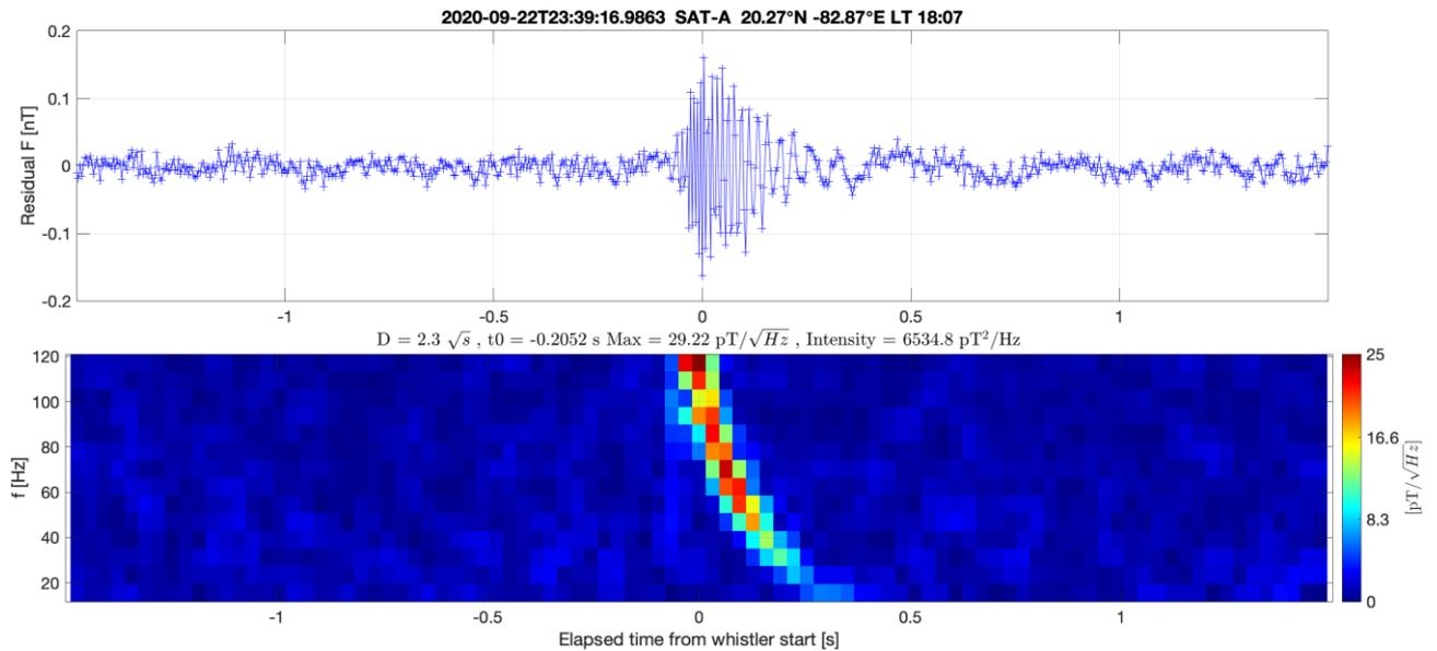
Figure 3-2 Example of strong whistler event recorded in burst data. Top panel: time series of magnetic field intensity, after removal of large-scale trends. Bottom panel: Power spectral density plot showing the frequency evolution of the whistler signals and the parameters computed for its characterization.
