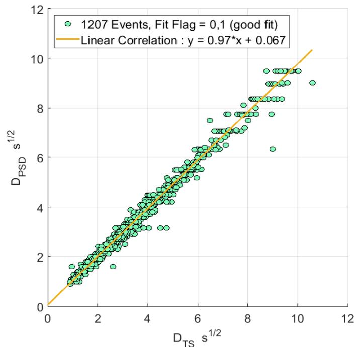
Figure 5-3 Comparison between dispersion obtained from a whistler wave fit on the ASM burst time-series  $D_{TS}$  and the dispersion  $D_{PSD}$  obtained from the PSD for 1207 selected events, for which the quality flag defined for the  $D_{TS}$  indicated a good fit.
