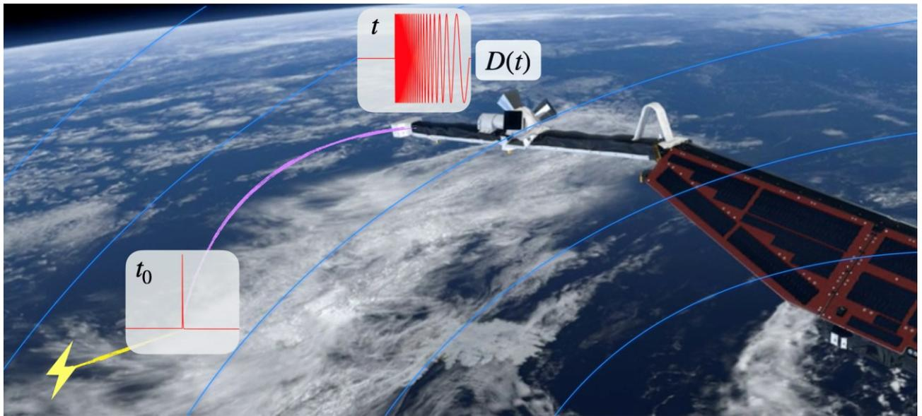
Figure 3-1 Schematic representation of the physical processes involved in the generation of a whistler signal detected by Swarm.  $t_0$  corresponds to the time when the lightning electromagnetic signal enters the ionosphere and  $t$  the time when it reaches Swarm and its dispersion is  $D(t)$ . The blue lines represent the Earth's magnetic field lines.
