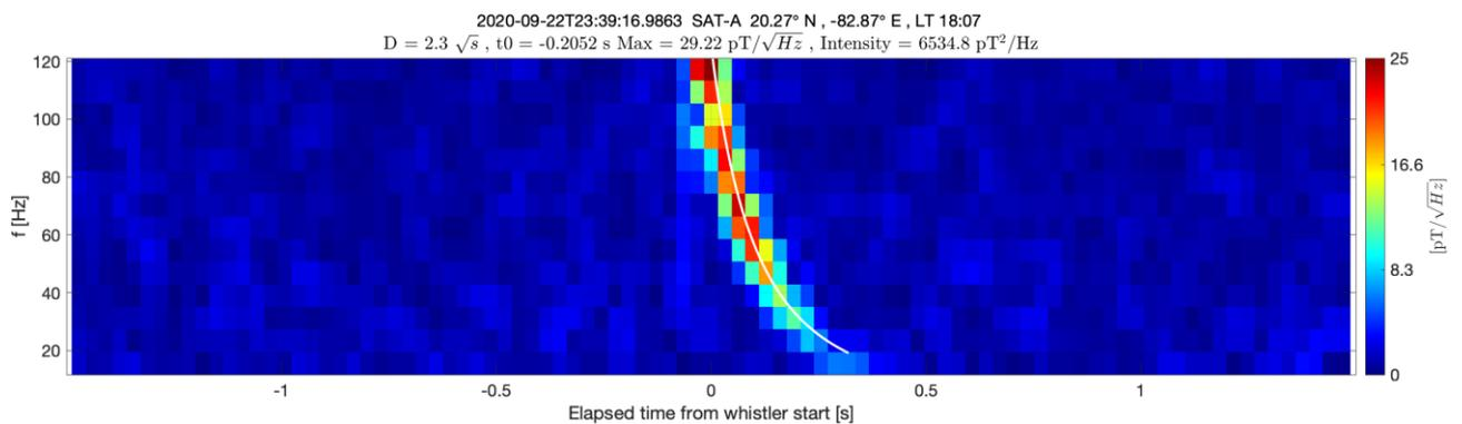
Figure 5-2 Example of whistler with the theoretical dispersion curve superposed in white. This curve is used to obtain the dispersion and timestamp values for the event.
