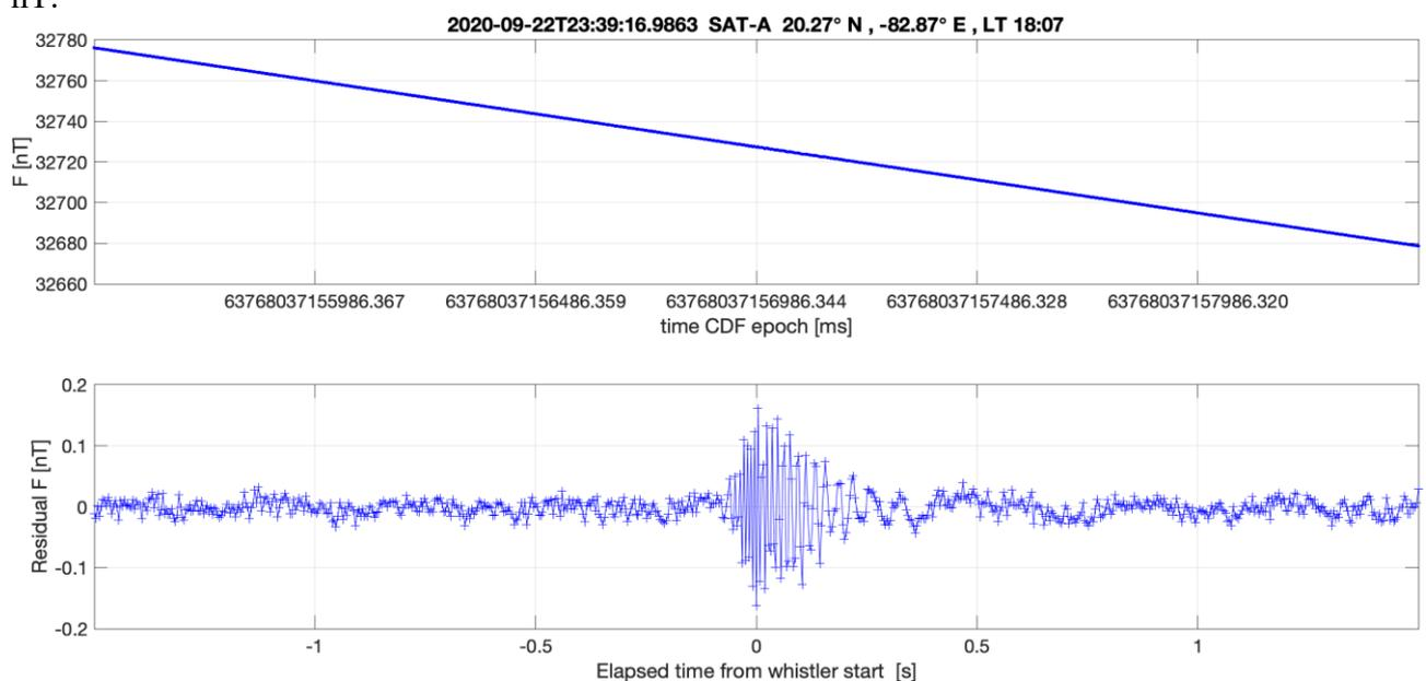
Figure 5-1 Example of large-scale trend removal for a whistler event. Top panel: ASM burst total intensity over a time window of 3 s. Note that the time scale following the CDF epoch scale is obtained combining `Timestamp` and `TimeFrac` variables. Bottom panel: the corresponding `F_analysed`; in this panel the time is shown relative to `Timestamp_Whistler`, indicated in the figure title in the form of a calendar date and UTC time.
