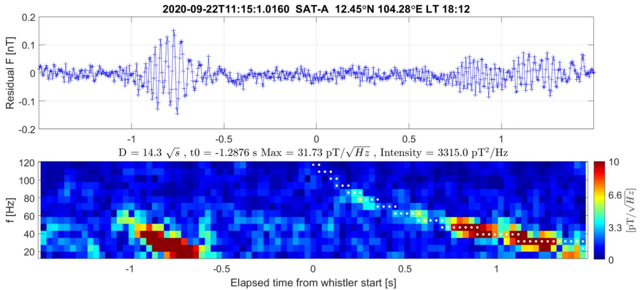
Figure 6-2 Example of whistlers occurring in rapid succession. The event identified with the white dots has a dispersion of  $14.3 \sqrt{s}$  and does not present a signature above 90 Hz. Its characterization is affected by ambiguity.
