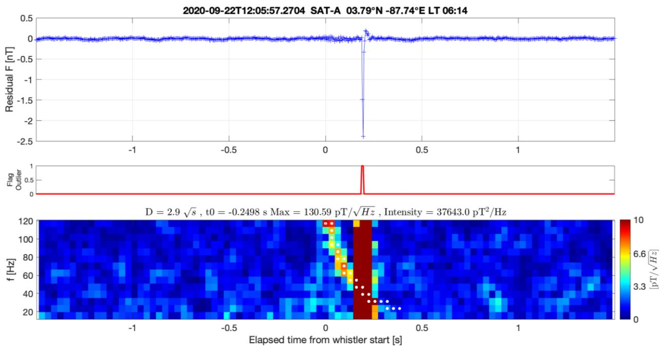
Figure 6-3 Example of outlier in ASM burst data occurring during a whistler event. The resulting Intensity value is unrealistically large. Top panel:  $F_{\text{analysed}}$  value. Middle panel: flag outlier. Bottom panel: PSD of the whistler event. The white dots indicate the PSD values that are used to compute the intensity.
