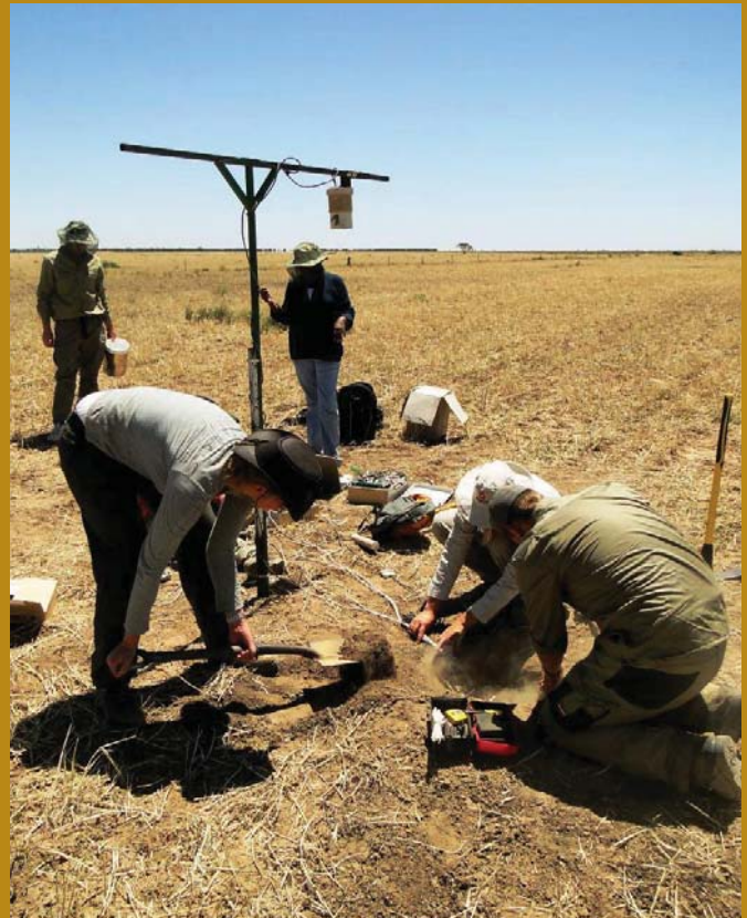
↑ Taking in situ soil moisture measurements during a five-week campaign in southeast Australia to validate SMOS data (Univ. Melbourne)
