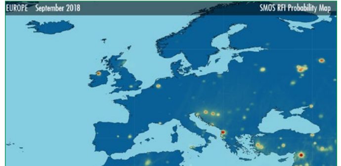
Figure-9: Map of Europe showing the probability of SMOS persistent RFI occurrences during September 2018. Credit: SMOS RFI team at ESA ESAC
