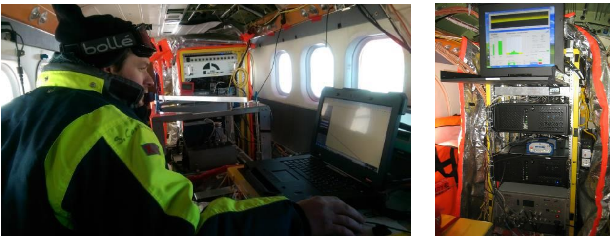
Fig. 3. Left: Forward look in of the cabin, with LCR gravimeter sensor and magnetometer and power conditioner rack unit; right: ASIRAS installation in the back of aircraft cabin.
