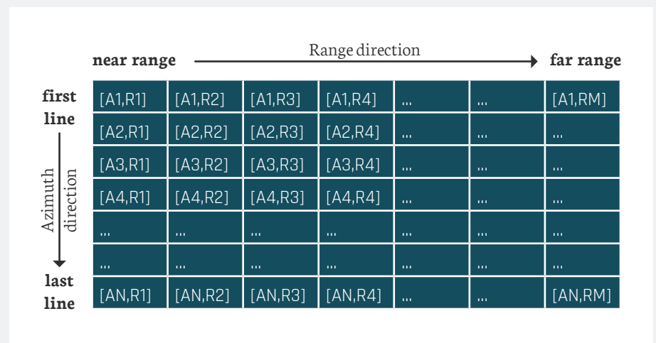
Figure 4. Complex SAR scene geometry in slant range
