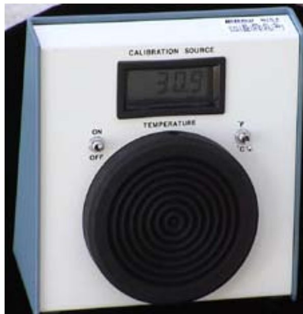
Figure 22 The infrared calibration source
