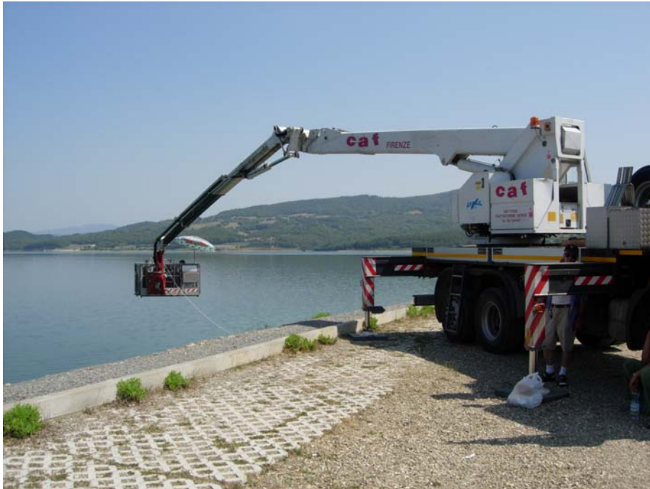
Figure 11 The experimental set-up for sky and water measurements
