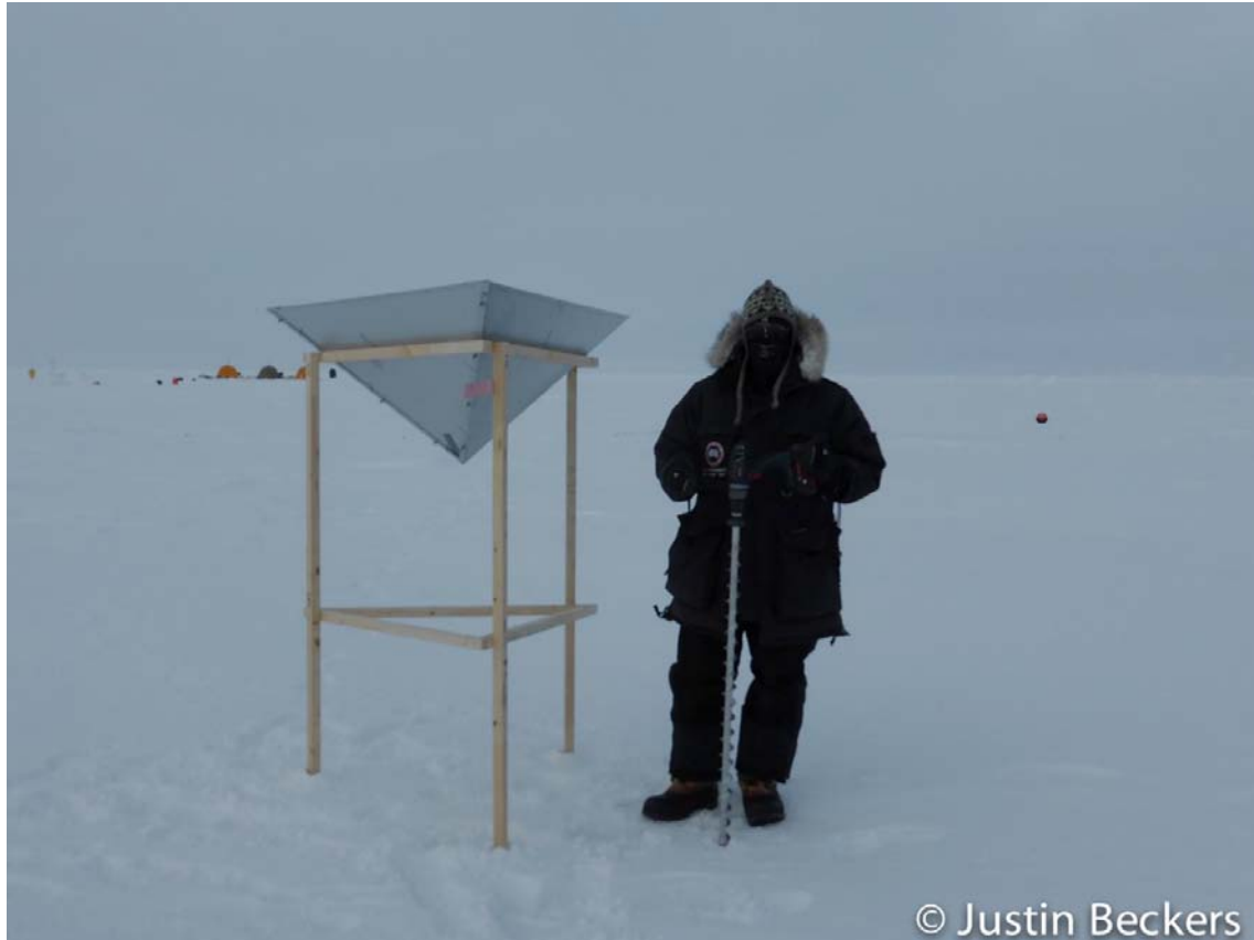
Figure 2: Christian Haas standing next to the East corner reflector at MIZ/ONR Camp 2.
