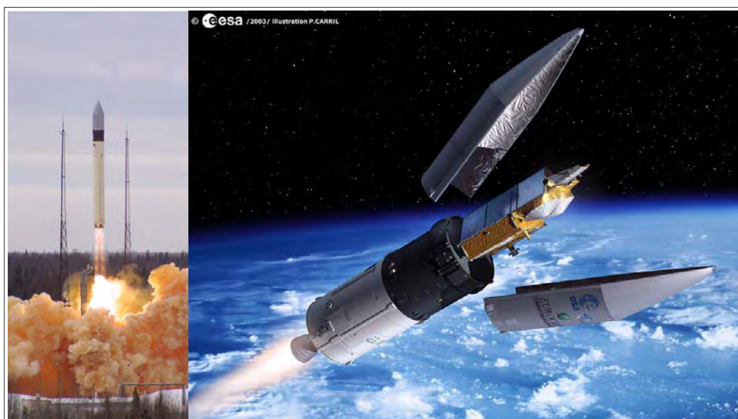
Figure 3.1–1 Left: the launch of GRACE on 17 Mar 2002 using a Rockot launcher. Right: an artists impression of the release of the fairing during the second-stage flight. The Breeze-KM upper stage is within the black cylinder between the satellite and the second stage.
