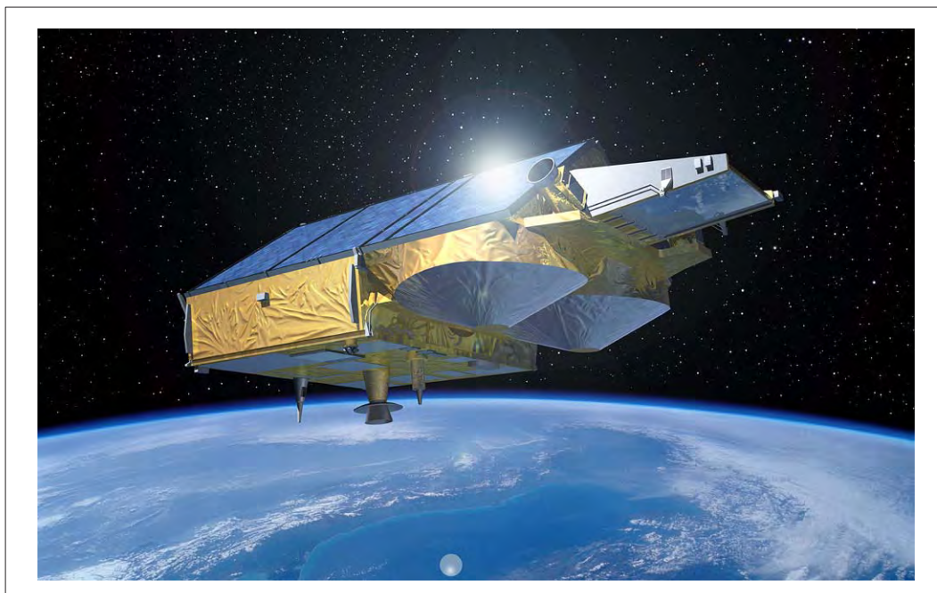
Figure 4.5-2 Perspective view of the CryoSat satellite, showing the thermal covers on the SIRAL antennas.
