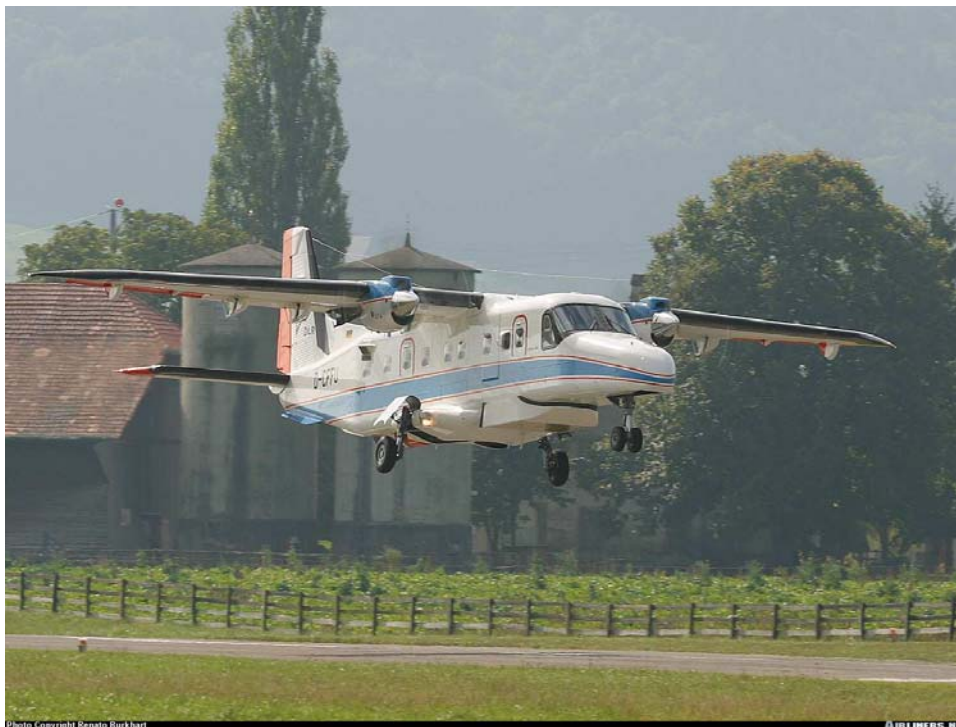
Figure 3.1: The E-SAR radar installed onboard a DLR DO 228 aircraft
