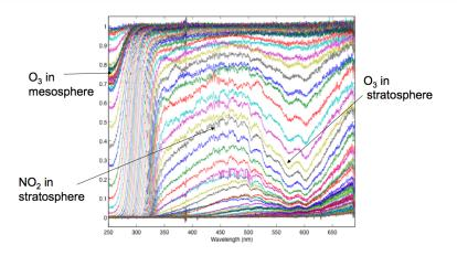
Transmission spectra measured by GOMOS at descinding altitudes from 100 km down to 5 km.
