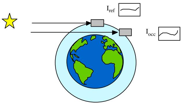
The diagram illustrates the principle of star occultation. A yellow star on the left has two light rays directed towards the Earth. One ray passes directly through the atmosphere above the Earth's horizon, labeled  $I_{\text{ref}}$  with a wavy line graph. The other ray is blocked by the Earth's atmosphere, labeled  $I_{\text{occ}}$  with a wavy line graph. The Earth is depicted with blue oceans and green continents.
