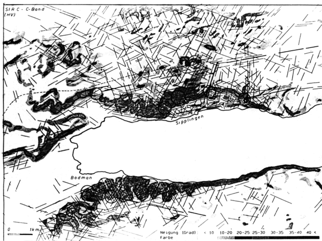
Figure 10: Slope gradient map of the northwestern Lake Constance area combined with the SIR-C C-band lineament map to delineate areas objected to slope failures
