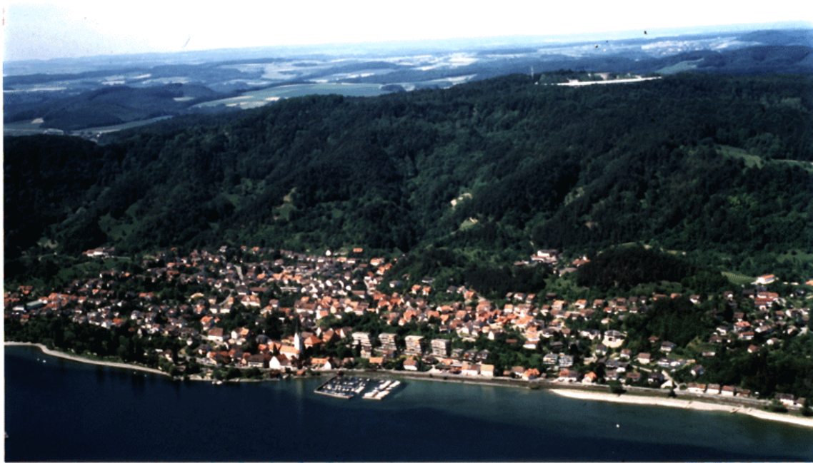
Figure 9: Aerial photograph - oblique view (to NW) from the northwestern Lake Constance area showing block movements of tertiary sandstones towards the lake near Sipplingen (Theilen-Willige, 31 May 1996)
