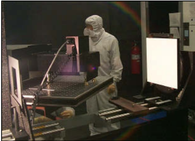
FEL-type standard lamp with diffuse reflectance standard to realize values of spectral radiance.
