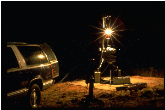
Irradiance standard lamp, calibrated for horizontal operation, for in situ calibration of downwelling solar irradiance instrument.
