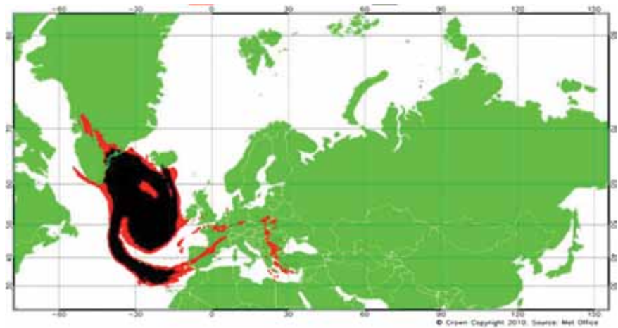
Fig 4. London VAAC modelled Eyjafjöll ash plume extension and concentration over Europe for 5 May 2010. Black areas indicate airspace where the ash concentration exceeds threshold values (no-fly zone) and red areas indicate airspace where ash might be encountered by aeroplanes. (UK Met Office)
