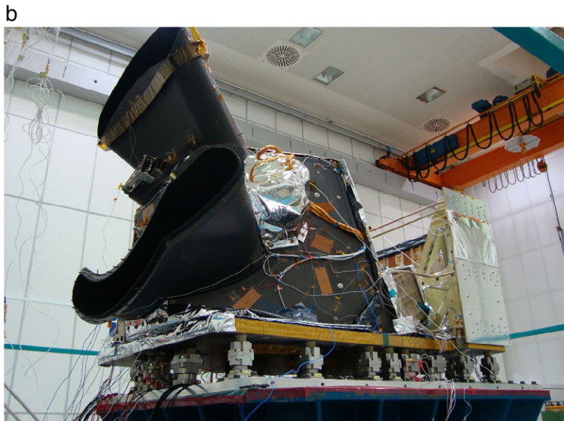
Fig. 7. (a) An overview of the Sentinel-3 Sea and Land Surface Temperature Radiometer (SLSTR) instrument highlighting principal components of the instrument design. (b) Photograph of the SLSTR Structural and Test Model (STM). (Credit: Selex-Galileo & Jena-Optronik)
