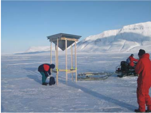
Figure 5.7-8 Picture of corner reflector over sea ice, pre-campaign in March/April 2004.
