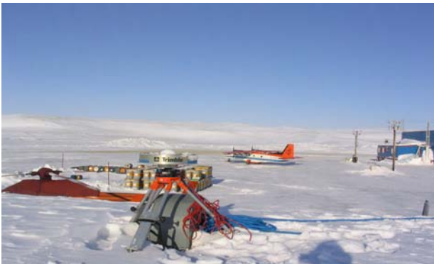
Figure 5.2-2 Resolute: DGPS ground station, antenna on top of the construction building (ca. 3 m above the runway) Receiver was powered by 110 V and was installed in the construction building. Data was named with RESU
