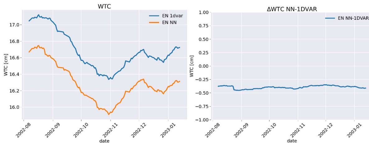
Figure 3-17 – ENVISAT: Daily global average monitoring of the WTC retrieved from the NN (orange) or the 1DVAR (blue) approach (left) and the differences between the two approaches (right). A 30-days moving average is applied to smooth the daily differences.
