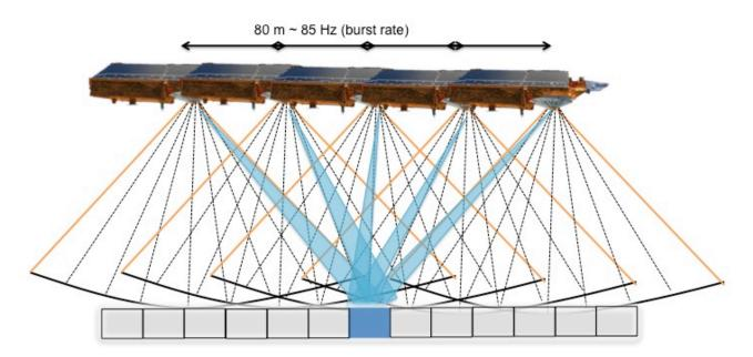
Figure 3: Geometry of multi-looking
