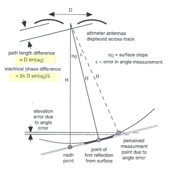
Figure 4: SARin mode across-track angle determination
