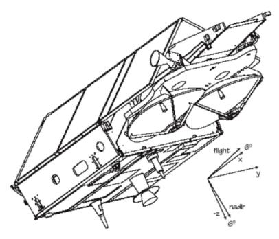
Figure 6: Satellite Reference Frame
