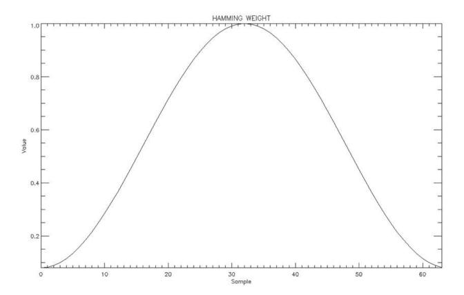
Figure 11: Hamming weighting function
