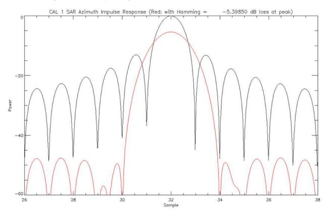
Figure 9: Comparison of AIR with and without Hamming window
