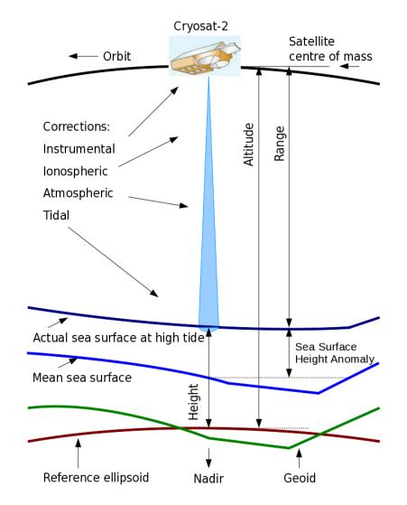
Figure 7: Basic altimetry terms and applicable corrections over open ocean
