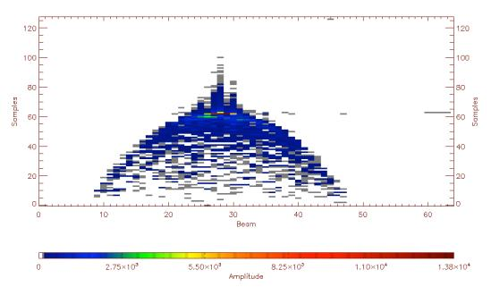
Figure 13: Azimuth FFT of a single burst with hamming: the nadir clutter is reduced
