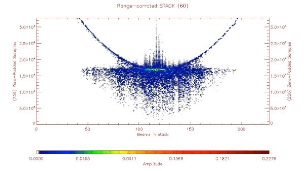
Figure 14: Stack 60 without hamming: here the parabola is the nadir clutter
