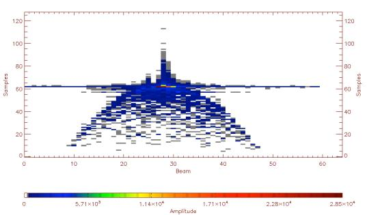
Figure 12: Azimuth FFT of a single burst: the nadir clutter is the 'line' in the middle
