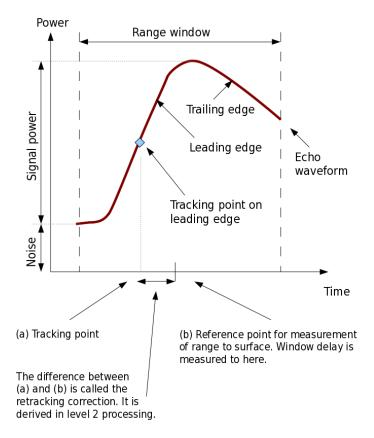
Figure 16: Idealised pulse-limited waveform in window
